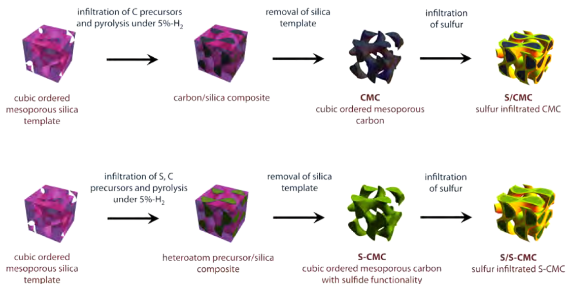
Figure 1. Preparation of cubic ordered mesoporous carbon (CMC) materials with and without sulfide functionality.
